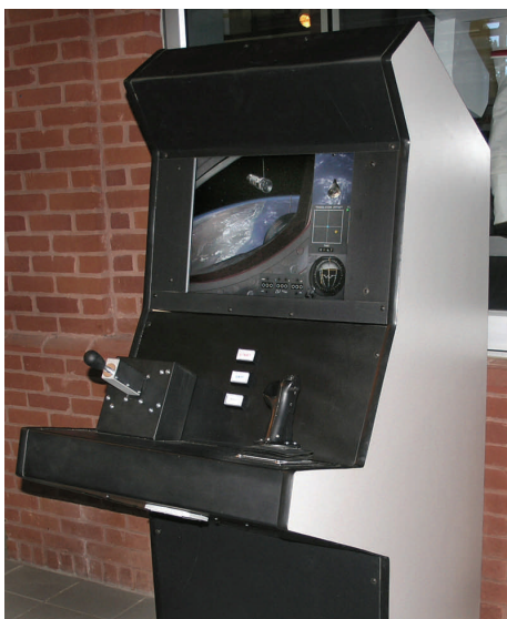
The Gemini Docking Simulator may be enclosed as a simple kiosk such as this exhibit at the Coca-Cola Space Science Center. Or you may choose to simulate a portion of the Gemini cockpit as well.
